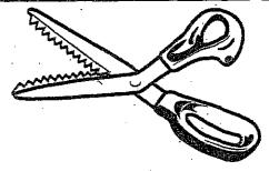
Cuts a zig-zag edge to prevent raveling. Makes a seam finish.
